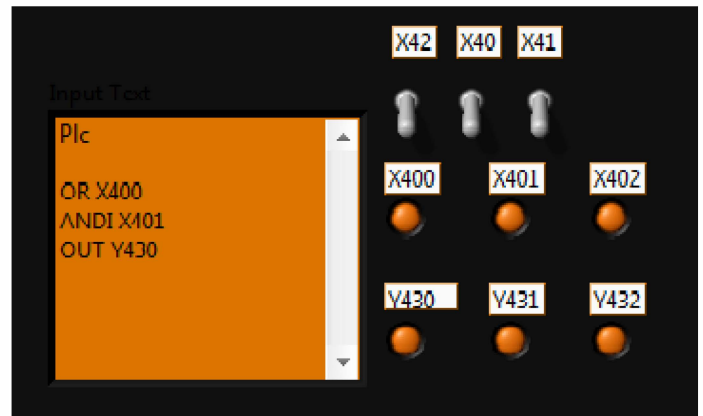
Figure 5. A screen shot from a sample STL command in the STL analyzer LabVIEW application
